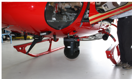
Plate 4 MX10 Fitted to AS350 Squirrel
